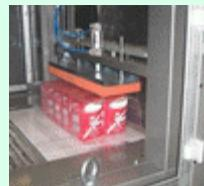
**Film presser roller unit** installed at the tunnel outlet it compacts the excess of film that remains on the sides of the package when total closure **of the package is required**
