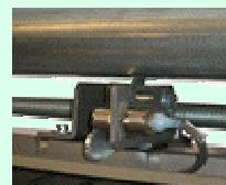
**Automatic upper and lower film spool centering system** by hand wheel.
