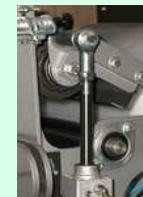
**Manual lifting** of the lower/upper spool joint in order to speed up changing.
